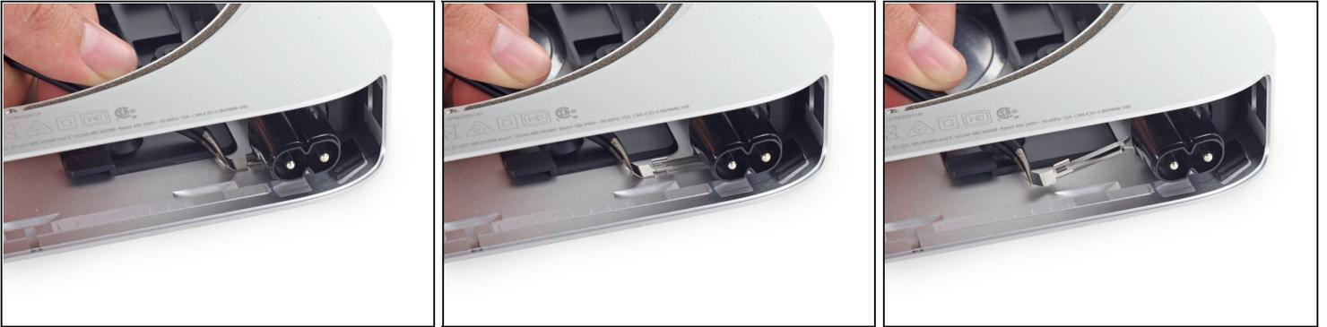
**i** The AC-in socket is secured with a small metal retaining clip.
