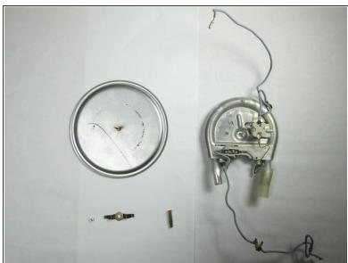
Pull the heating element off of the heating plate.
