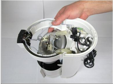
Using the larger plastic opening tool, gently push the tubing off of the one-way valve. (If the tubing is being stubborn and won't come off, run the metal spudger around the inside of the tubing to free it up.)
