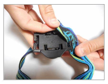
Pull the bottom of the righthand strap through the middle bracket on the mount. The strap should now be completely free from the mount.
