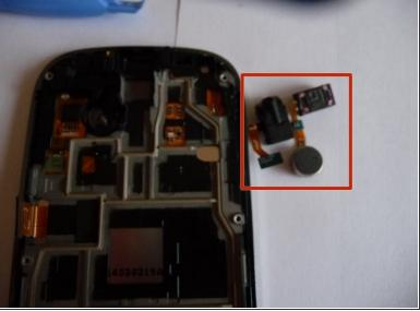
• Use a plastic opening tool to pry up the headphone jack, vibrator, and earpiece speaker assembly.
