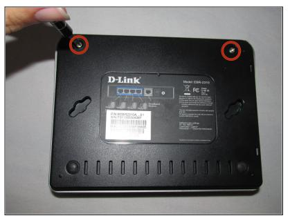
• Using a Phillips #2 screwdriver, remove the two top screws.
