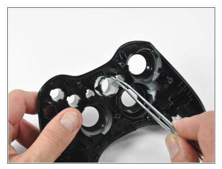
Using a pair of tweezers, remove the LED ring from the front panel.
