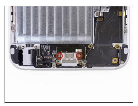
Remove the two 3.3 mm Phillips #00 screws securing the metal bracket to the Lightning connector assembly.
