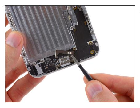
Use a pair of tweezers to lift and remove the metal bracket out of the iPhone.
