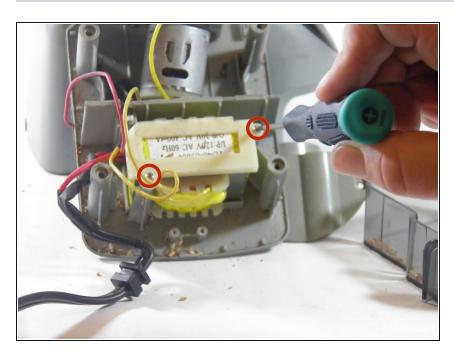
Using a Phillips00 screwdriver, remove the two 10.42mm screws on the plastic frame securing the power component.
