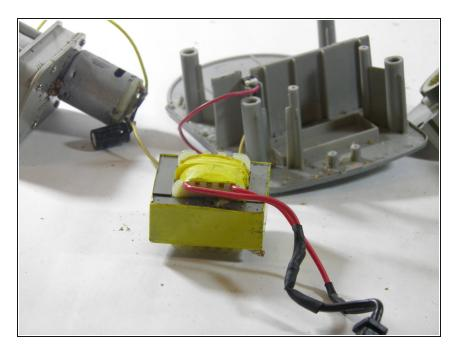
Carefully lift out the power component from the panel.
