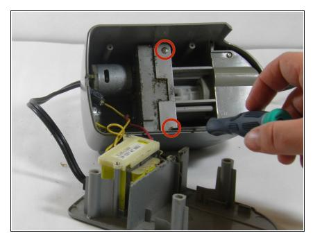
Using a Phillips00 screwdriver, remove two 10.3mm screws from the middle section of the top panel.
