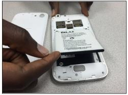
• Remove the back cover by lifting at the notch towards the bottom of the phone. Use your fingernail to pry up.
