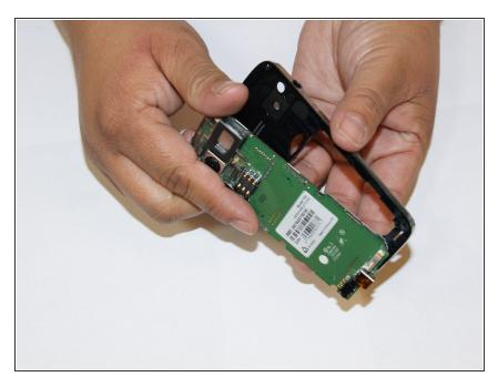
The back casing is removed by taking the motherboard and back casing and pulling them apart.
