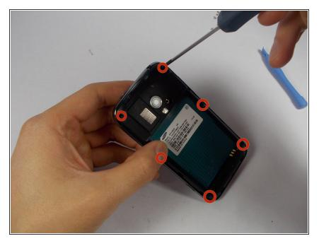
• With a small phillips-head screw driver, remove the six screws holding the back panel in place.
