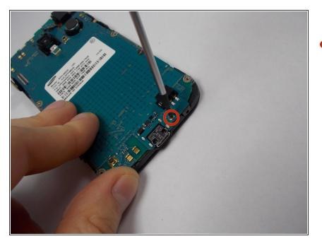
Use a philips-head screwdriver to remove the single screw on the bottom of the phone. Located to the right of the charging port.
