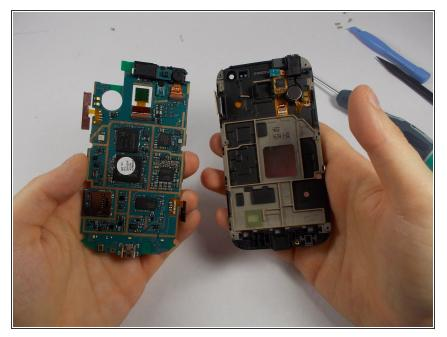
• Lift the motherboard upwards separating it from your screen.
