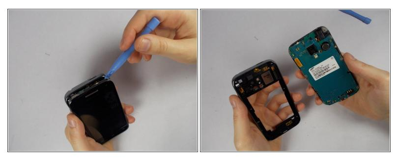
• Use the pry tool to pry the back panel from the rest of the phone. Pry from the edge closest to the screen for simplicity.
