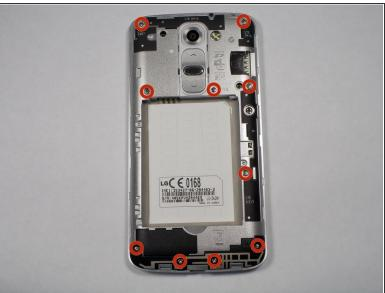
Locate 10 screws and remove each one using a screw driver.
