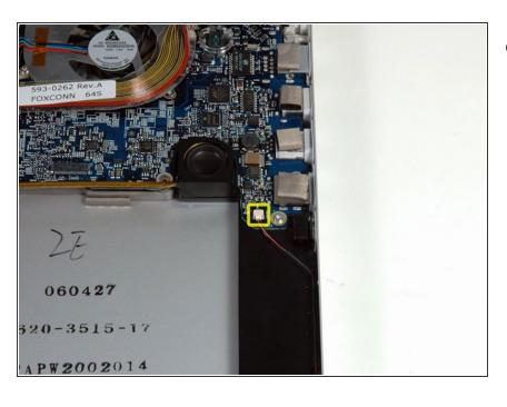
Disconnect the PRAM battery cable from the bottom right corner of the logic board.
