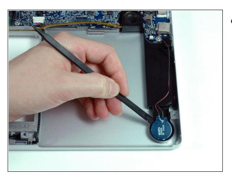
Use a spudger to pry up the PRAM battery from its housing on the left speaker assembly.
