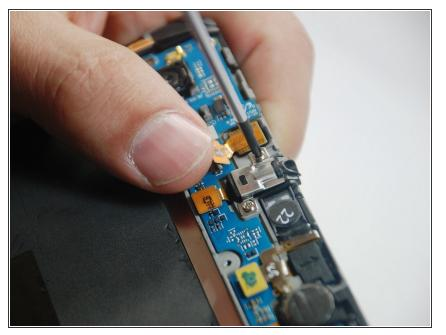
Use the Phillips #00 screwdriver to remove the 2 screws that secure the audio jack in place.
