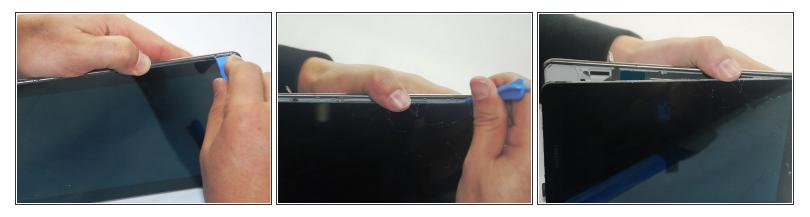
Insert the prying tool between the glass screen and the silver binding. Pry around the screen until the screen is separated from the back of the tablet.
