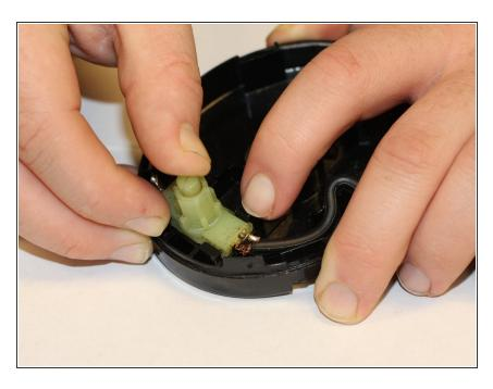
The trigger button is held in with light tension clips. Gently pry them back to release.
