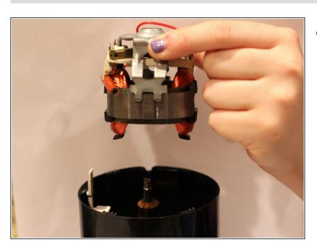
Remove the motor from the shell.
