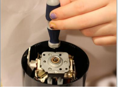
Using a Phillips screwdriver, remove the two screws holding the motor in place.
