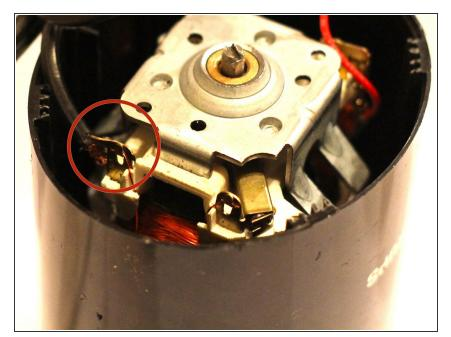
Desolder remaining contact point from the plug cord
