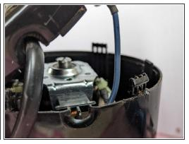
Wedge the spudger between the flat side of the E-clip and the outside wall of the slot. Then, loosen
