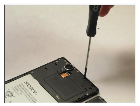
Using the Phillips #00 Precision screwdriver, take out 8 silver screws (3.15mm) and 5 gold screws (3.9mm) for a total of all the screws attached to the flat plate. 3 of the gold screws are located at the top of the phone and the other 2 screws are located at the bottom of the phone.
