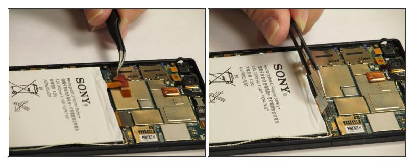
Using the Tweezer, carefully pry open the corresponding chips that are attached to the battery as shown. Then using the spudger, pry the battery away from the phone and watch out for the sticky substance keeping the battery to the phone.
