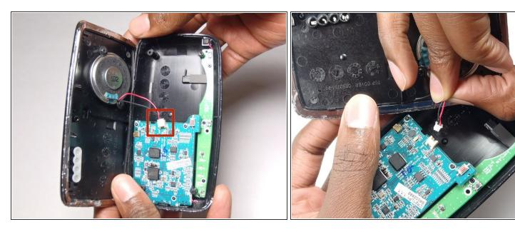
Carefully detach the wire running from the speaker to the motherboard by unplugging it from the white socket.
