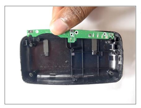
Remove the status display by lifting it off of the back plate.
