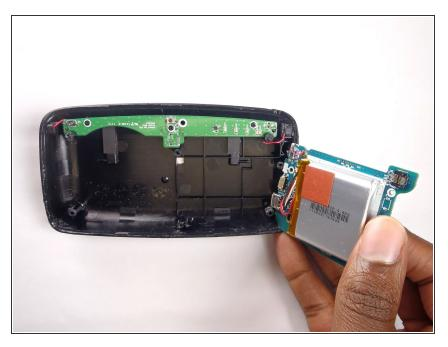
Remove the motherboard from the device by lifting it up from the back plate.
