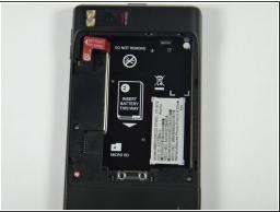
Pull up on the red battery release tab and pull the battery out of the phone.
