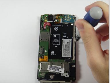
• Remove these nine screws using a T-3 torques. These screws should be 2.40 mm in length
