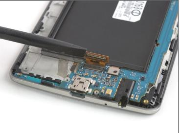
• Use a spudger to pry up and disconnect the display flex cable.
