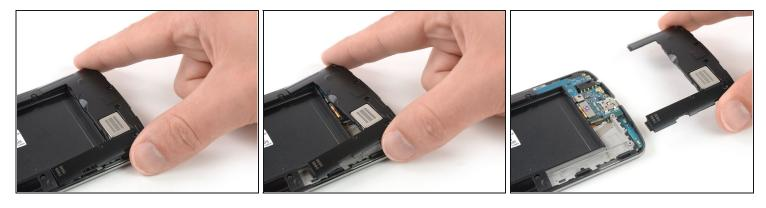
• Carefully remove the plastic panel including the loudspeaker by gently pulling it away from the phone assembly.
