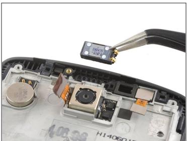
⚠ During removal of the earpiece speaker, remove it together with the foam gasket underneath.
