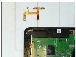
Now that the contacts are no longer attached, you can use either tweezers or your fingers to grasp and lift contacts vertically off of the device.
