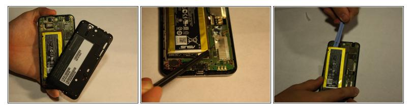
• Once the Battery has been successfully removed, move on to the step 2.
