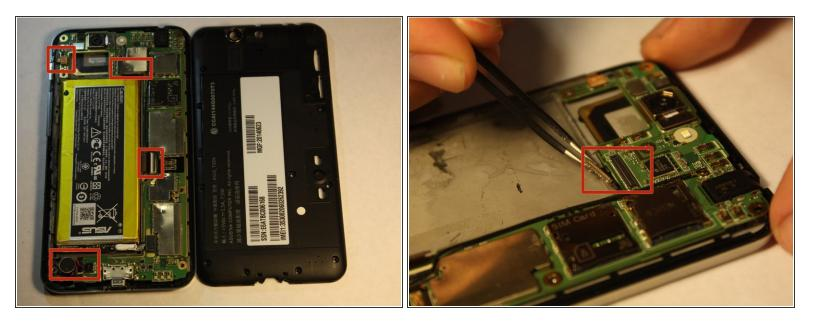
• Disconnect the marked strips from the logic board using the tweezers.
