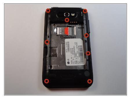
• Use a Phillips #00 Screwdriver to remove all eight 4mm screws.
