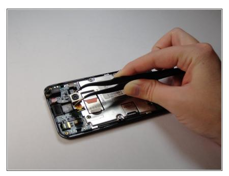
• Use tweezers to remove the camera, you will need to use some force as it is glued on.
