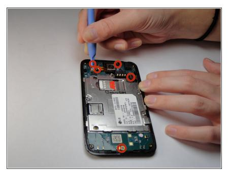
Pry off the circled tabs using a plastic opening tool to release the motherboard.
