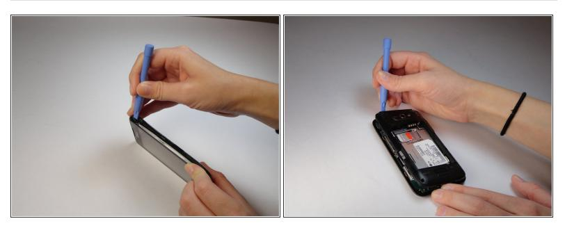
• Use a plastic opening tool to remove the back trim by working around all of the edges.
