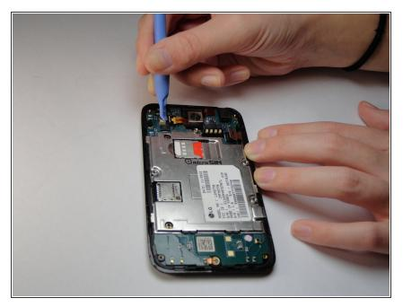
• Pry slightly underneath the tab attached to the camera until it pops off.
