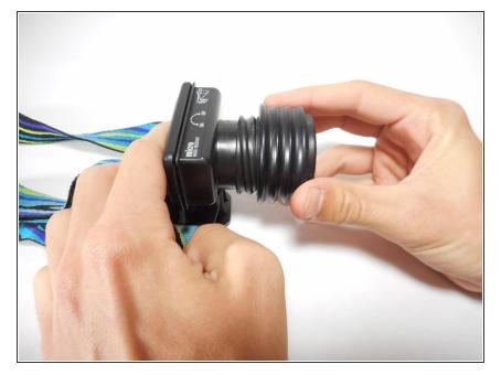
Attach the new lens piece by firmly pressing the open end of the lens piece onto the battery housing.
