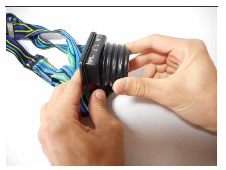
Secure the new lens piece onto the battery housing by turning the lens piece clockwise (right) until the headlamp turns on. You have just successfully replaced the lens piece.
