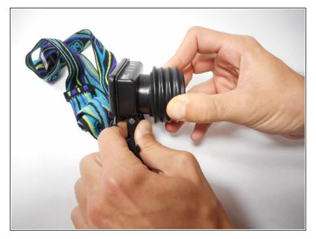
Remove the damaged lens piece by rotating the lens piece counterclockwise (left) until the lens piece is fully extended.
