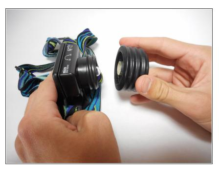
• Remove the extended lens piece by firmly pulling the lens piece away from the battery housing. Take care
