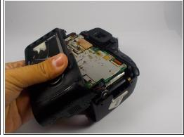
Use a plastic opening tool to separate the rear case from the camera.
