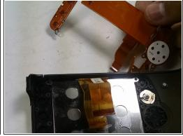
Use a plastic opening tool to separate the LCD and metal plates from the casing.
