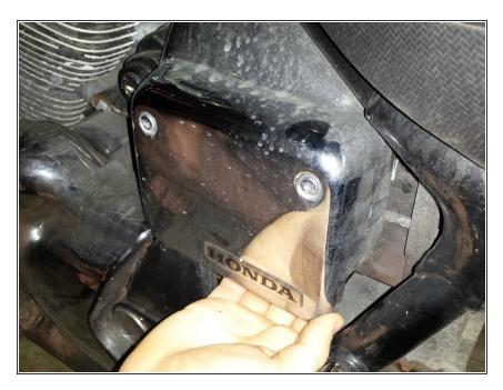
Remove the plastic covering, located on the left side of the bike, by pulling the piece straight off the bike.
