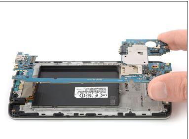
Grab the top section of the motherboard and carefully lift it out of the phone.
