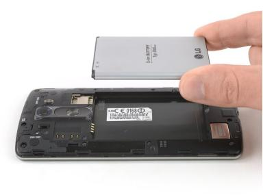
Lift the battery out of its recess and remove it.
