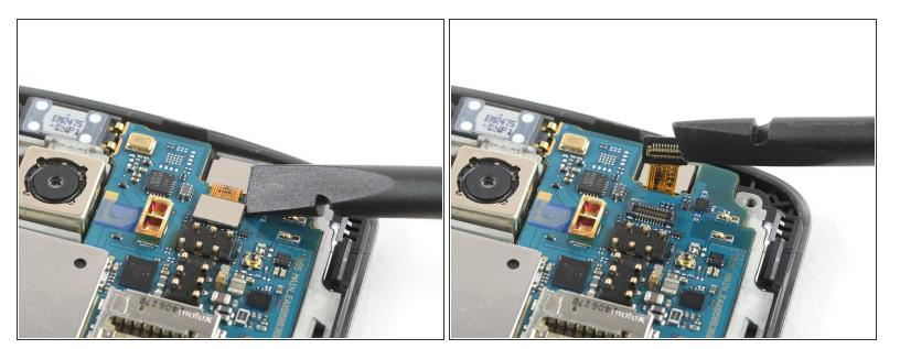
Use a spudger to pry up and disconnect the front camera flex cable.
