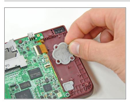
Lift the rubber pad off the back of the D-pad.
