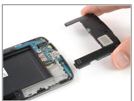
Carefully remove the plastic panel including the loudspeaker by gently pulling it away from the phone assembly.
