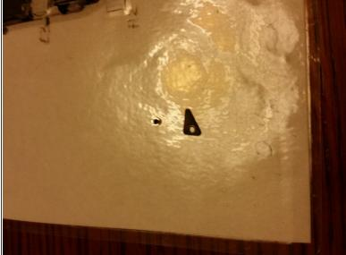
Remove 2 X screws and triangular washer
