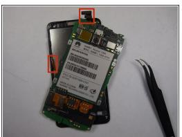
Carefully detach the LCD and speaker ribbons from the Motherboard using the pliers
