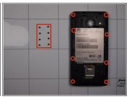
Remove the 8 screws on the back and place them on the magnetic mat
