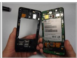
Pull of the back cover using the plastic opening tool
