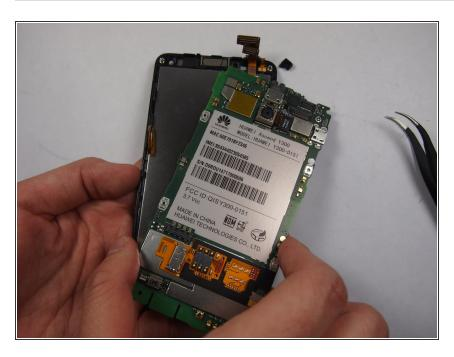
replace the motherboard with a new one and re-attach the ribbon wires to the motherboard
