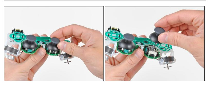
Pull the analog stick covers straight up off the joystick posts attached to the motherboard.
