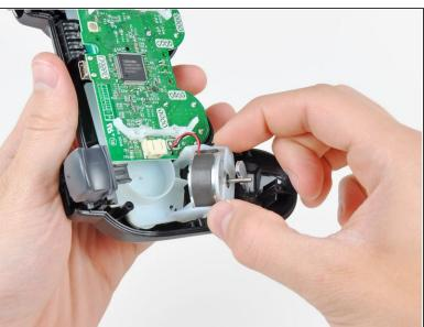
Pull the vibration motor retainers away from the front cover to dislodge the motherboard assembly.
