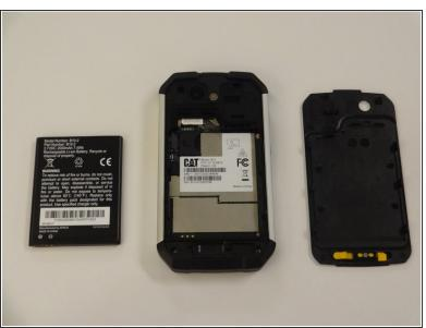
Place index finger at the top edge of the battery and gently lift upwards. The battery will slide cleanly out of the phone. The new battery can be inserted where the old one was. The phone can be reassembled by following these steps in reverse.
