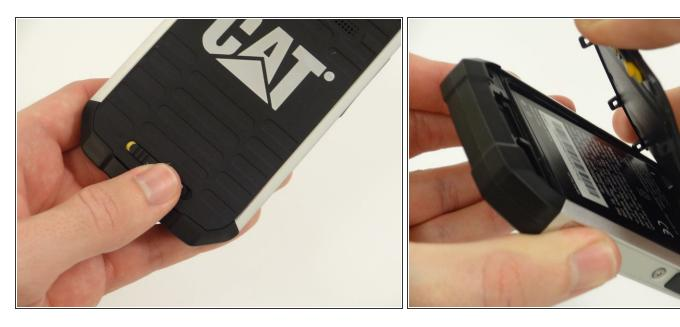
Remove the back covering by gently lifting upwards from the bottom of the back covering. The back will snap off and the battery is exposed.
