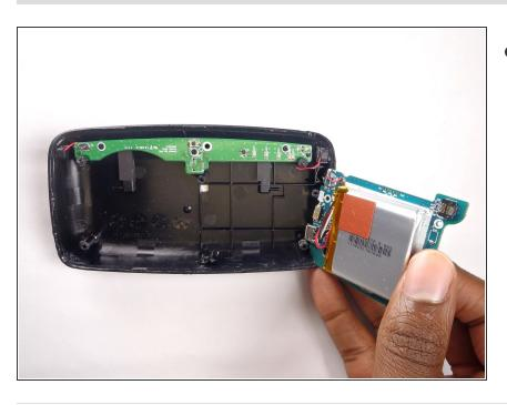
Remove the motherboard from the device by lifting it up from the back plate.
