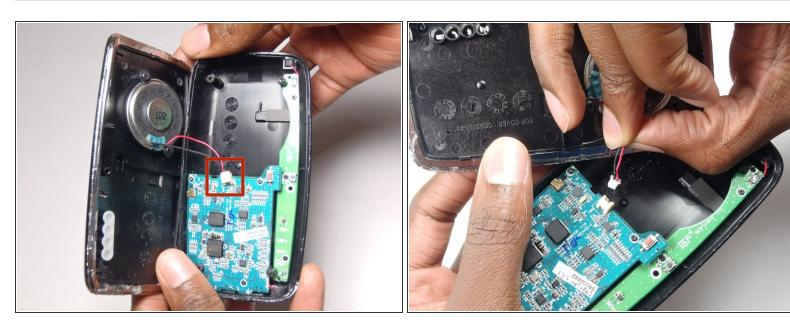
Carefully detach the wire running from the speaker to the motherboard by unplugging it from the white socket.
