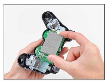
Lift the battery off the motherboard for enough clearance to access the battery connector.
