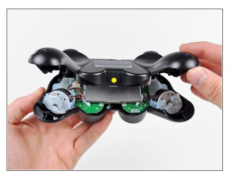
Press on the rear cover between the analog sticks and slightly lift the lower edge of it away from the rest of the controller.
