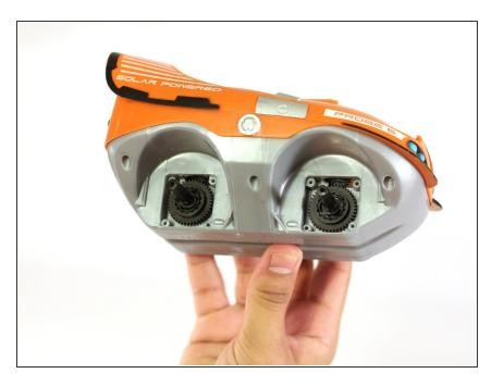
Pry open the two gear covers on both sides.
