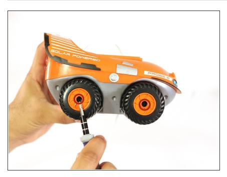
Remove both 8.0 mm Phillips #1 screws, one for each wheel.
