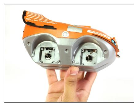
Pull the driving gears off the axles by sliding them off the axles and exposing both axles.
