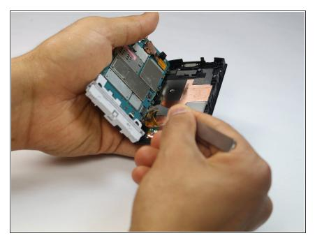
Carefully detach the flex cable using a pair of tweezers.
