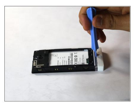
Remove the bottom cover of the phone using the plastic opening tool.
