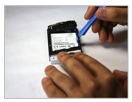
Carefully remove the back cover using the plastic opening tool.
