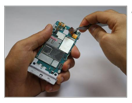
Use the tweezers to detach the flex cable to remove the camera.
