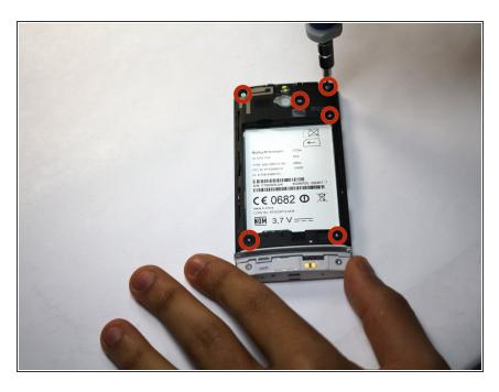
Remove the five 5.47mm and one 5.18mm Torx head screws using a Phillips #0 screwdriver.
