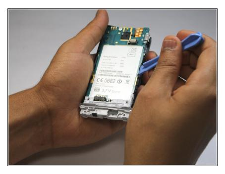
Pry up on the right side of the motherboard using the plastic opening tool.
