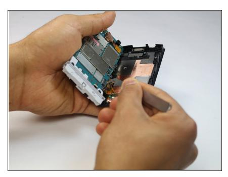
Carefully detach the flex cable using a pair of tweezers.
