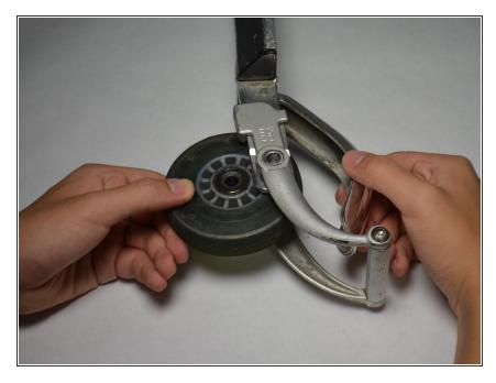
Turn the JD Razor 2000 on its side as shown. Slowly remove the back wheel by pulling it out at a perpendicular angle to the scooter base.
