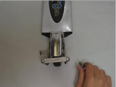
Remove the bolt from the right side and the bearing from the left.
