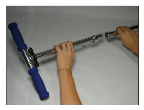
After disassembling the Quick-Release Lever, the T-Bar is removable
