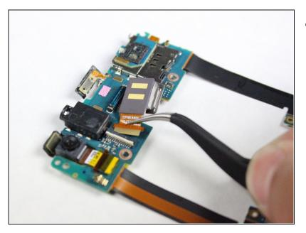
Use your tweezers to remove the rear-facing camera from the camera board.
