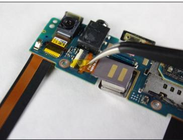
• Use your <u>tweezers</u> to gently pull off the two pieces of yellow tape in the center of the camera board.
