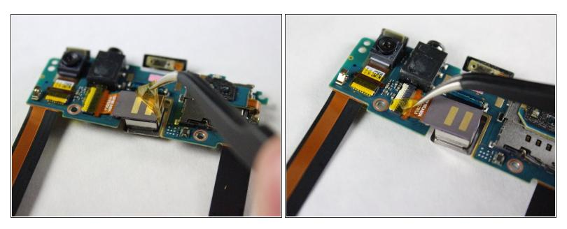
Use your tweezers to gently pull off the two pieces of yellow tape in the center of the camera board.
