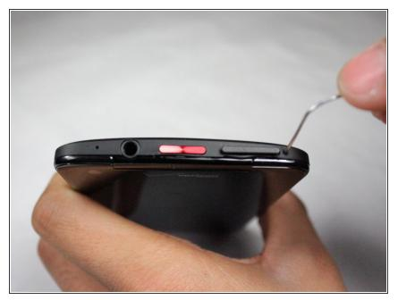
Poke a paperclip into the hole to the right of the SIM Card Tray. The SIM Card Tray will automatically pop out.
