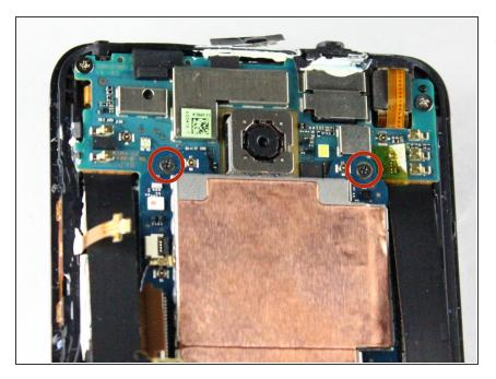
Use a Phillips #000 screwdriver to remove the two 3.9mm screws on top of motherboard.
