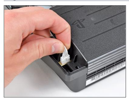
Pull the DC-Out cables straight up to lift their connector up and out of its socket on the power supply.
