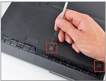
• Use the flat end of a metal spudger to pry up the seven screw covers around the edge of the lower case.
