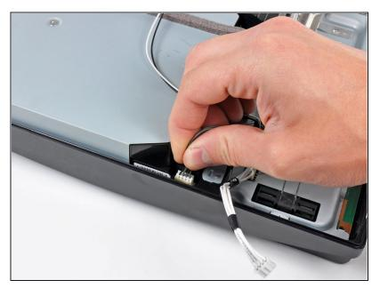
Pull the Blu-ray power cable straight up to lift its connector out of the socket on the Blu-ray drive.
