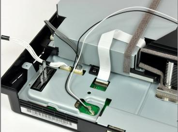
(i) If present, remove the pieces of tape securing the cables to the body of the Blu-ray drive.
