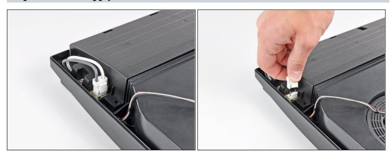
• Squeeze the AC inlet connector's locking mechanism and pull straight up to disconnect it from the power supply.
