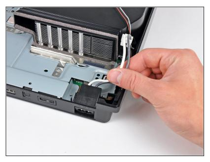
Pull the AC-In cables upward to remove the AC inlet from the lower case.
