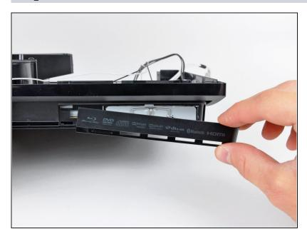
Slide the hard drive bay cover toward the right side of the lower case, then pull it away from the front edge to remove it from the PS3.
