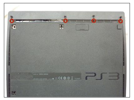
Remove the four 13.3 mm T8 security Torx screws beneath the Blu-ray drive opening. (Some models may only have three screws)
