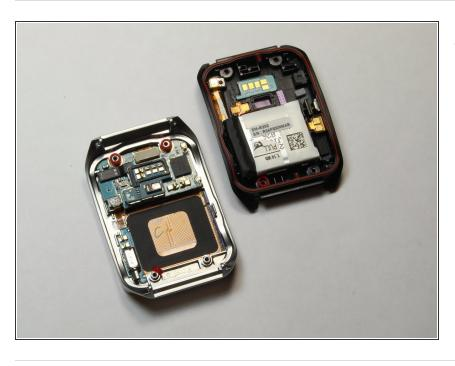
Lay both halves of the watch body assembly face down (with internal components facing up).
