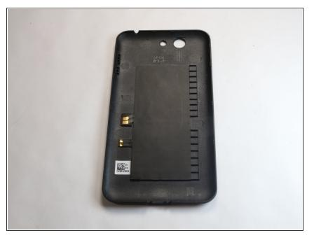
Replace the back cover with the new one; the antenna is integrated with the back panel.
