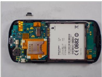
• When the inner back cover is off, locate and remove the power button.
