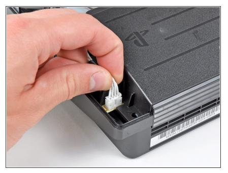
Pull the DC-Out cables straight up to lift their connector up and out of its socket on the power supply.
