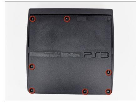
Remove the seven 37 mm Phillips screws securing the top cover to the lower case.
