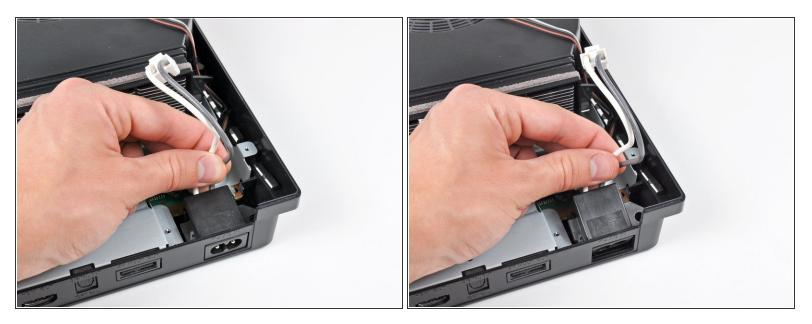
• Lift the AC inlet cables straight upward to remove the AC inlet from the lower case.
