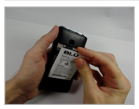
Place new battery with the correct orientation in place of the old one.
