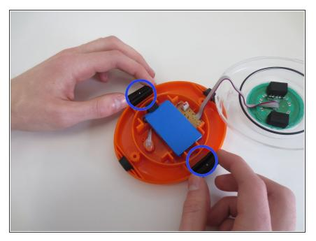
• Remove both ends of the strap from the orange casing by pulling up.
