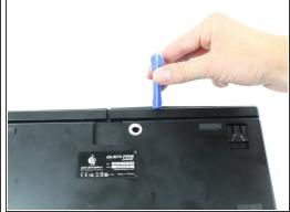
Wedge a plastic opening tool between the rear plate and rim of the keyboard and slide it through the circled areas to separate the plastic hooks that mount the rim to the rear plate.
