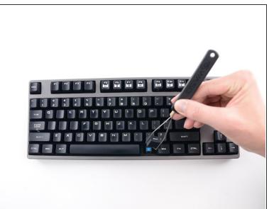
Remove the keycap of the key whose switch you'd like to replace by following the <u>small keycap</u> replacement guide or large keycap replacement guide.
